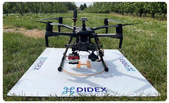
To create high-quality multispectral maps for an agribusiness in an area with dynamic weather conditions, Drone Imagery & Data Expert (DIDEX) turned to the new MicaSense RedEdge-P multispectral sensor used in combination with Measure Ground Control software for flight mission planning. The sensor's panchromatic sensor allows pansharpening that increases the resolution of its five multispectral bands to enable 3D multispectral mapping which was crucial for this project.
